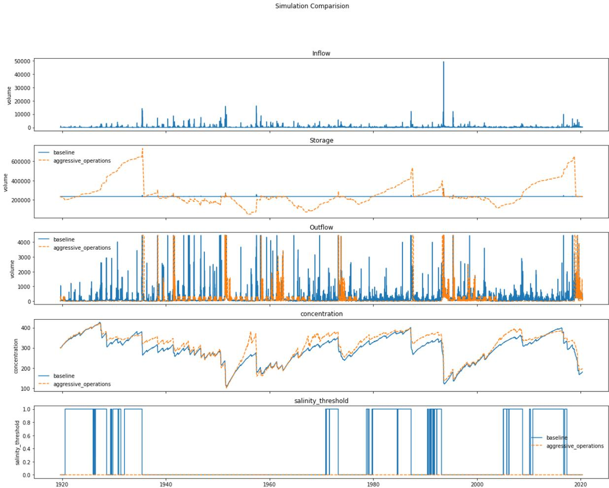
**Figure 24. Wilson Lake “aggressive” conceptual operational scenario simulation results**
