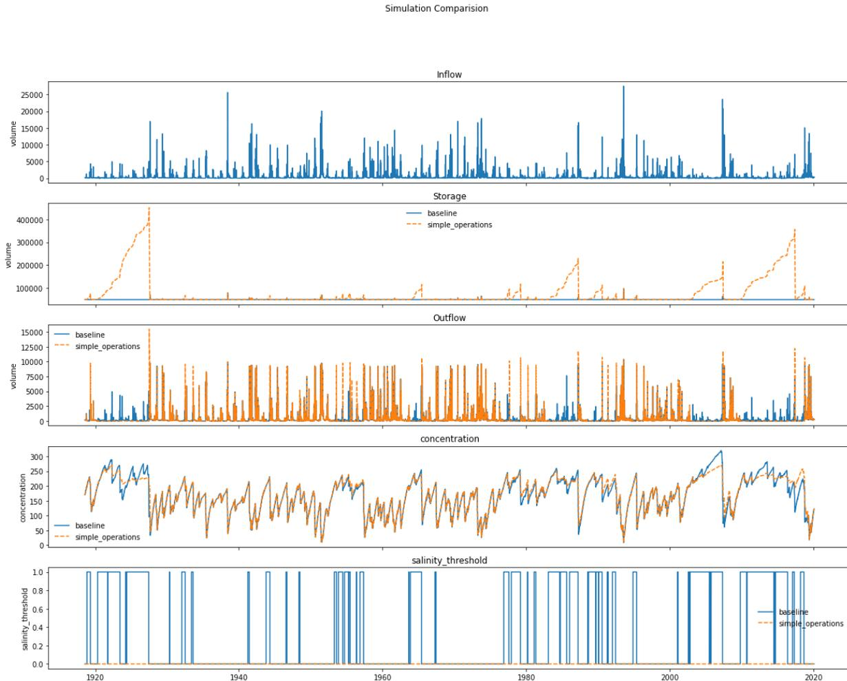
**Figure 23. Kanopolis "simple" conceptual operational strategy simulation results**
