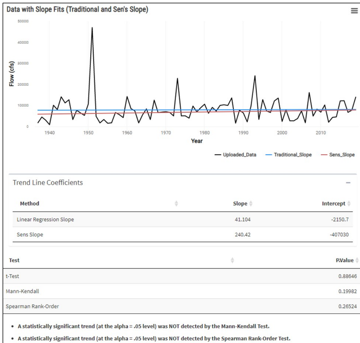
Figure 26. Lecompton Gage Trend Analysis Results from Time Series Toolbox (1937-2019)
