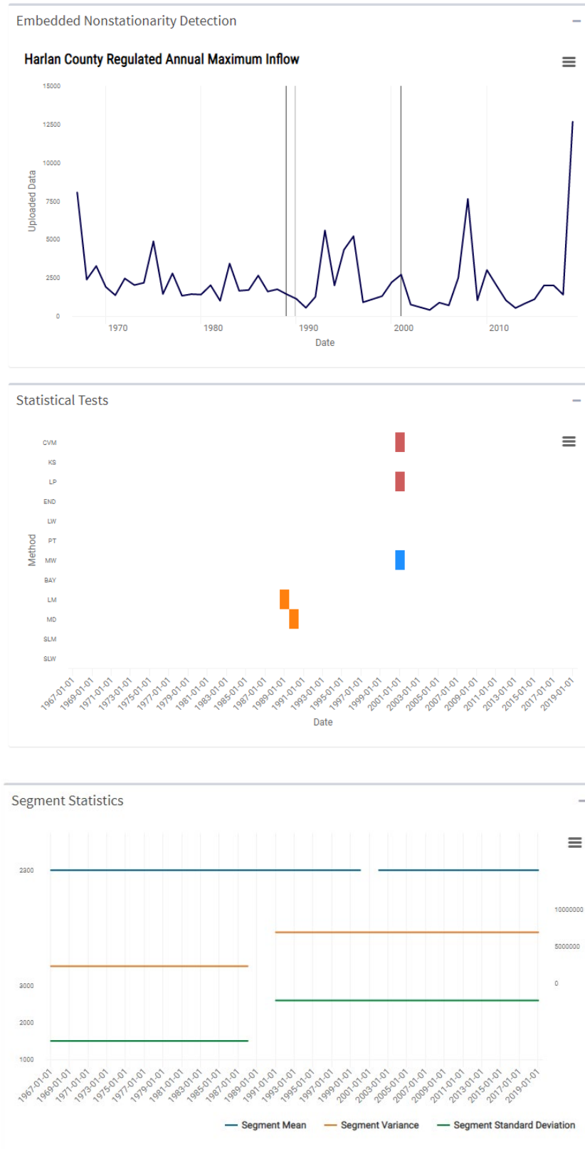
Figure 35: Nonstationarities Detected in Harlan County Lake Regulated Inflows (1967-2019), CPM Method sensitivity adjusted to 500
