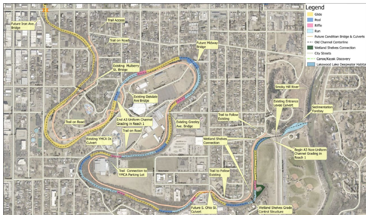
Figure 2-1 – Measures and their location (southern portion)
