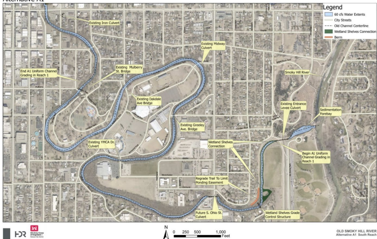
Figure 5-1. Alternative 1, Reach 1 – South Reach
