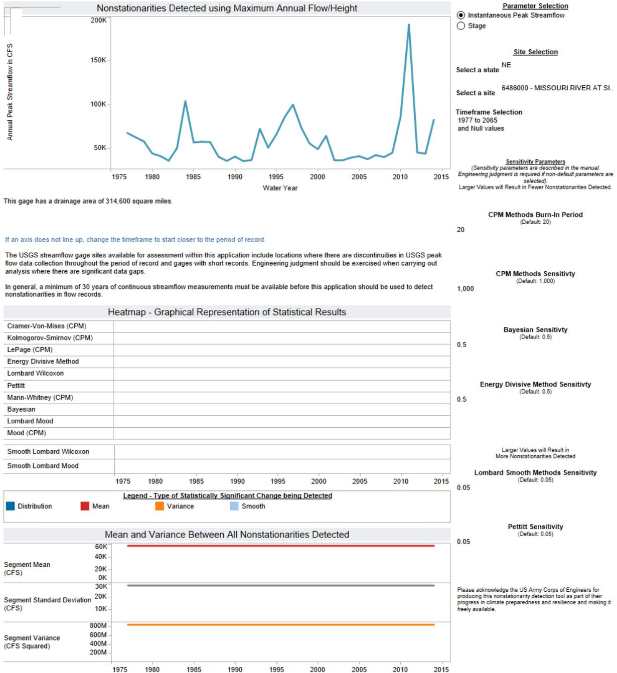
**Figure 30. NSD Output for USGS Gauge 06486000 Missouri River at Sioux City, IA**
