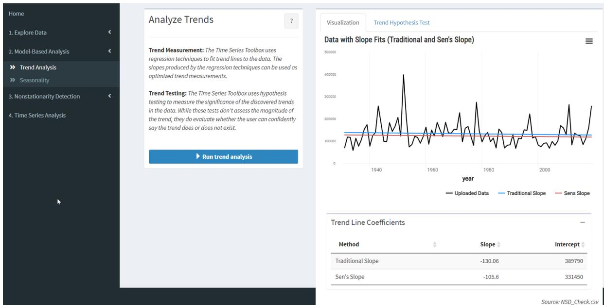
**Figure 133. Time Series Toolbox Trend Analysis Output for Bend Dam 7-day NRNI Peak Streamflow Time Series**
