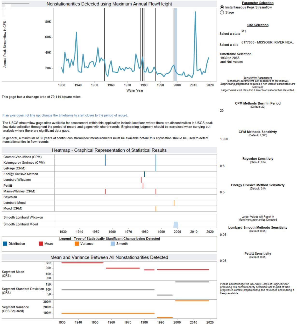
**Figure 34. NSD Output for USGS Gauge 06177000 Missouri River near Wolf Point, MT**
