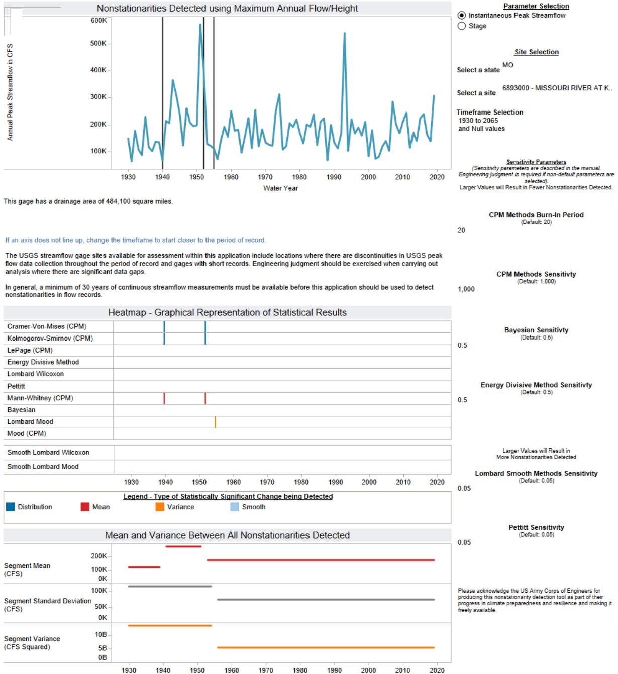
**Figure 40. NSD Output for USGS Gauge 06893000 Missouri River at Kansas City, MO**
