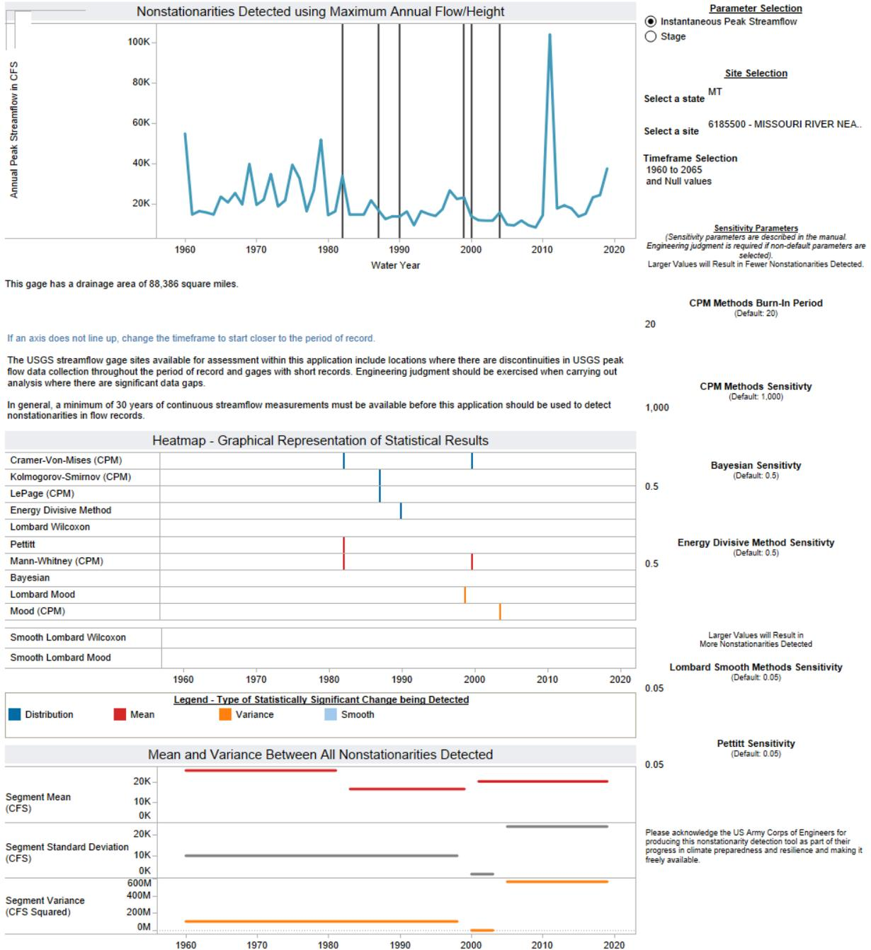
**Figure 32. NSD Output for USGS Gauge 06185500 Missouri River near Culbertson, MT**
