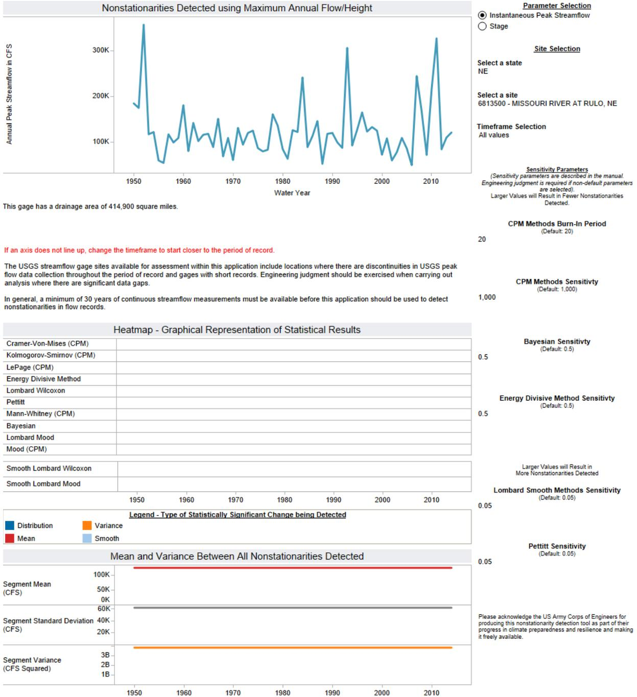
**Figure 36. NSD Output for USGS Gauge 06813500 Missouri River at Rulo, NE**
