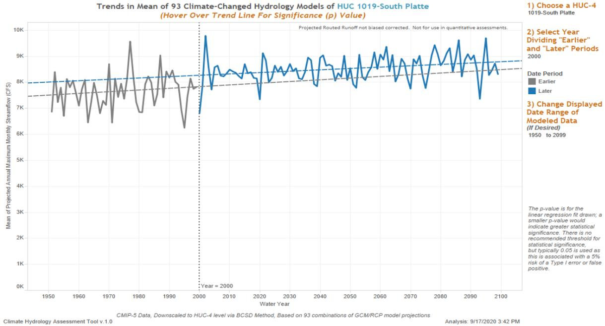
**Figure 29. Linear Regression of Mean Projected Annual Maximum Monthly Flow for HUC 1019 South Platte**
