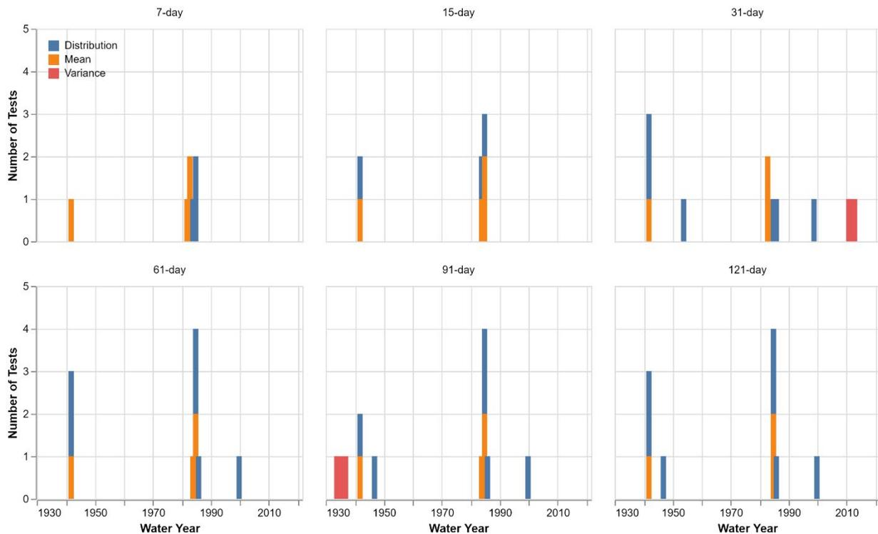
**Figure 43. Fred Robinsons Bridge Nonstationary Change Detection Points for n-day Durations Ranging Between 7 and 121 days**
