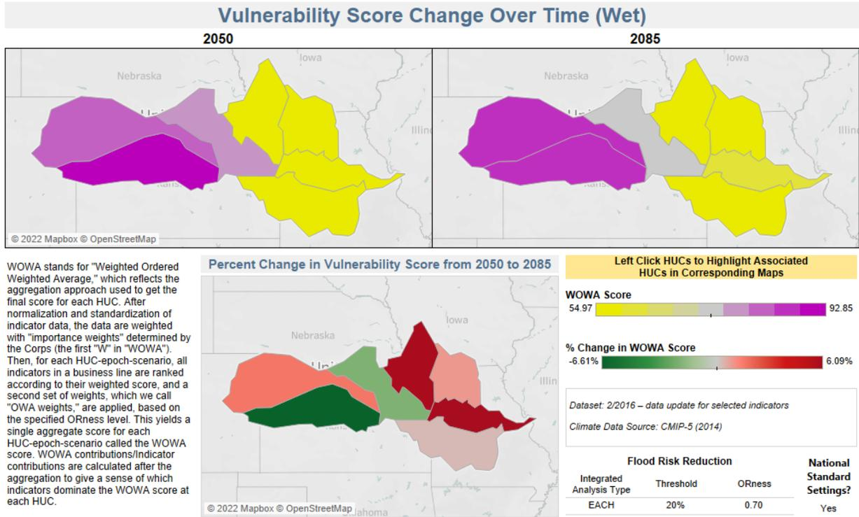
**Figure 28. NWK VA Tool Flood Risk Reduction Vulnerability Score Over Time for the Wet Scenario**
