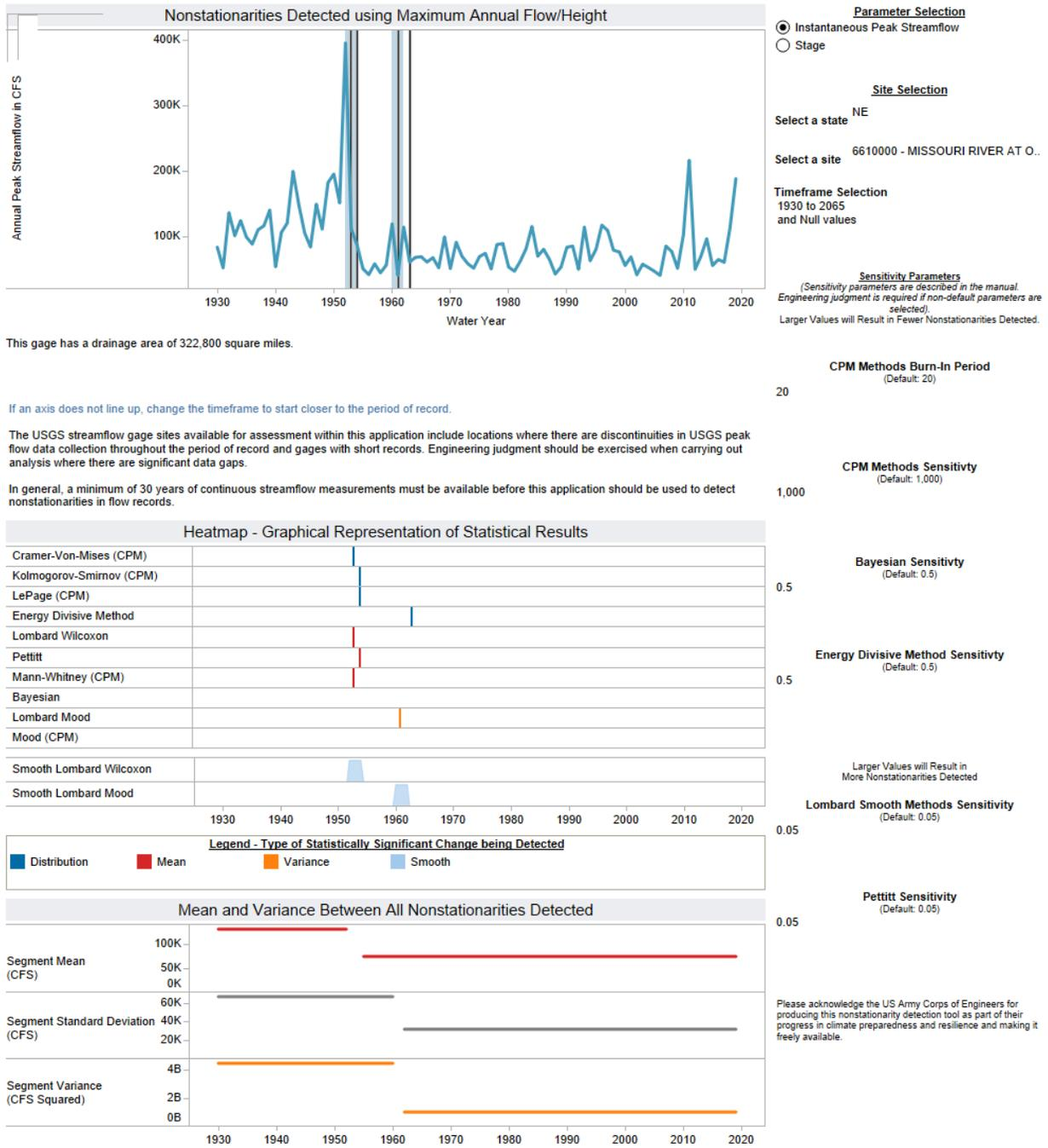
Figure 29. NSD Output for USGS Gauge 06610000 Missouri River at Omaha, NE
