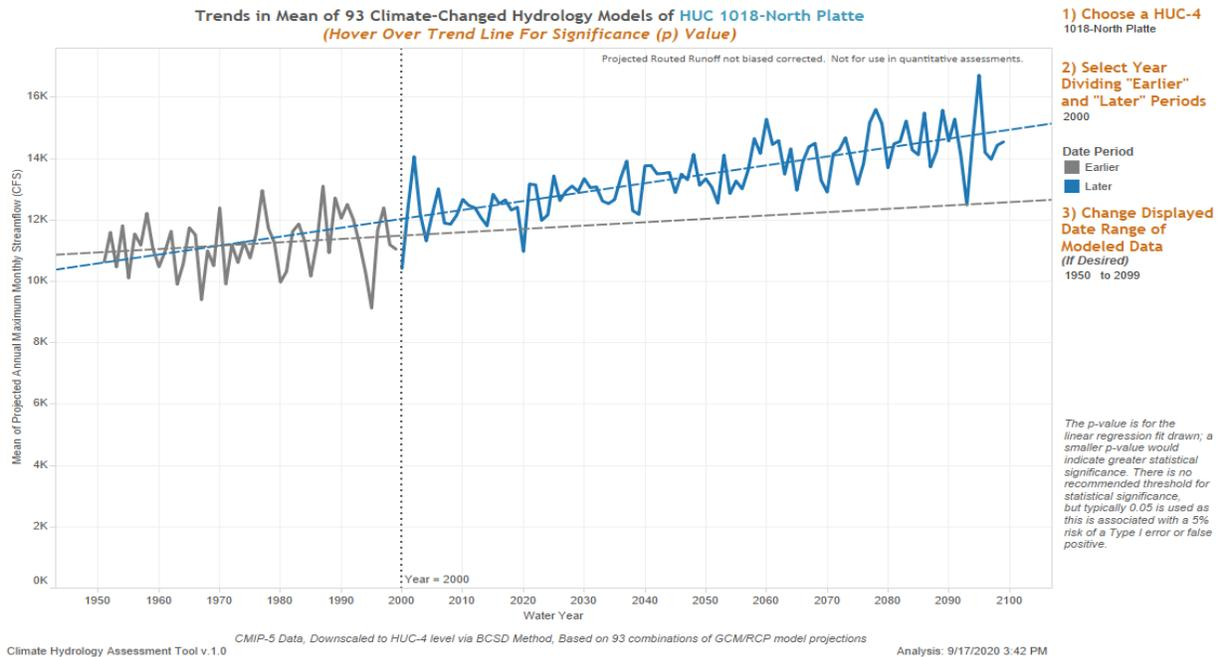
**Figure 28. Linear Regression of Mean Projected Annual Maximum Monthly Flow for HUC 1018 North Platte**
