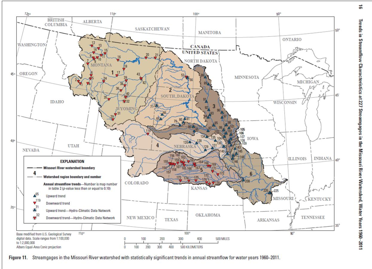
**Figure 3. USGS Streamgages in the Missouri River Basin with Statistically Significant Trends in Annual Peak Streamflow for Water Years 1960 – 2011 (Norton et al. 2014)**
