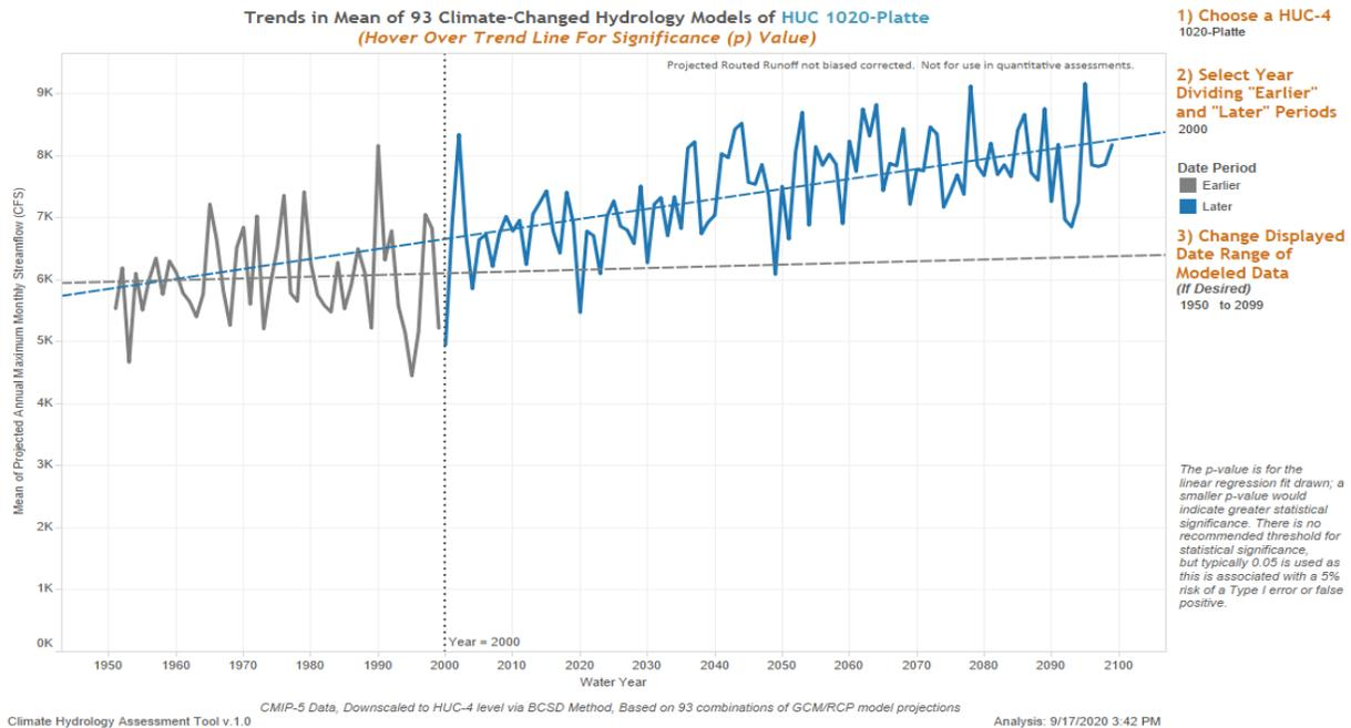
**Figure 30. Linear Regression of Mean Projected Annual Maximum Monthly Flow for HUC 1020 Platte**
