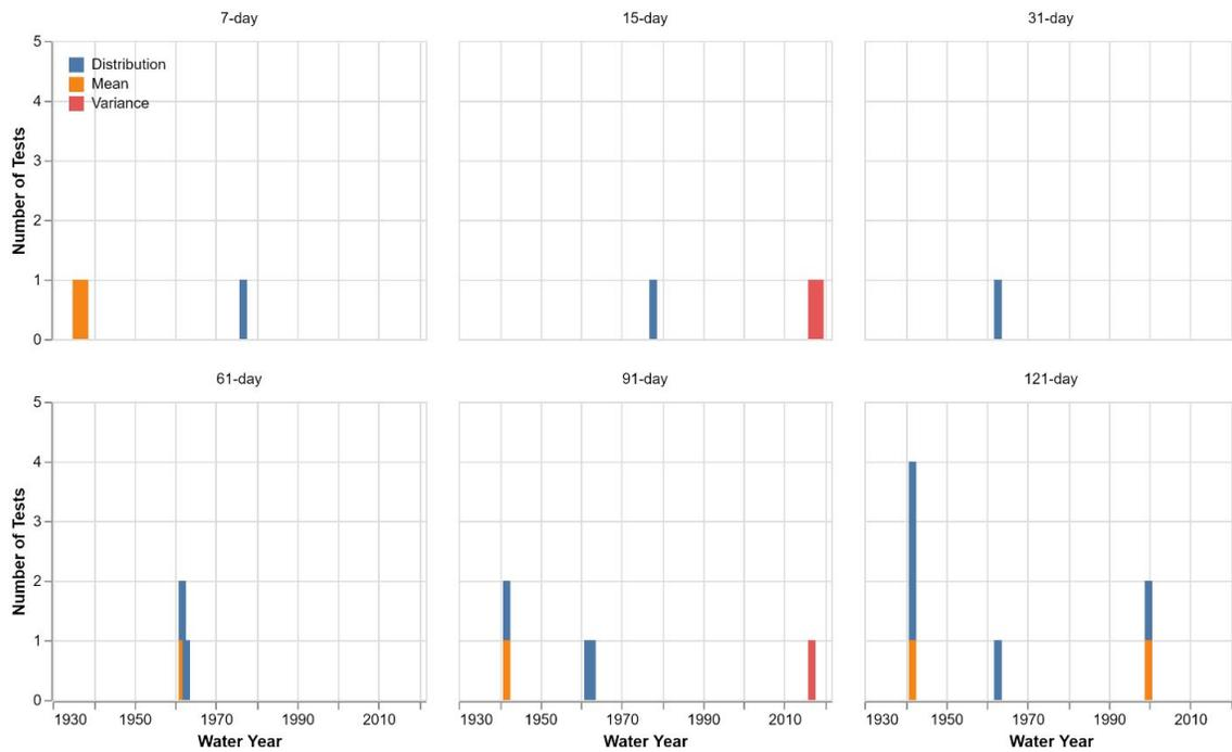
**Figure 53. Ft. Randall Nonstationary Change Detection Points for n-day Durations Ranging Between 7 and 121 days**
