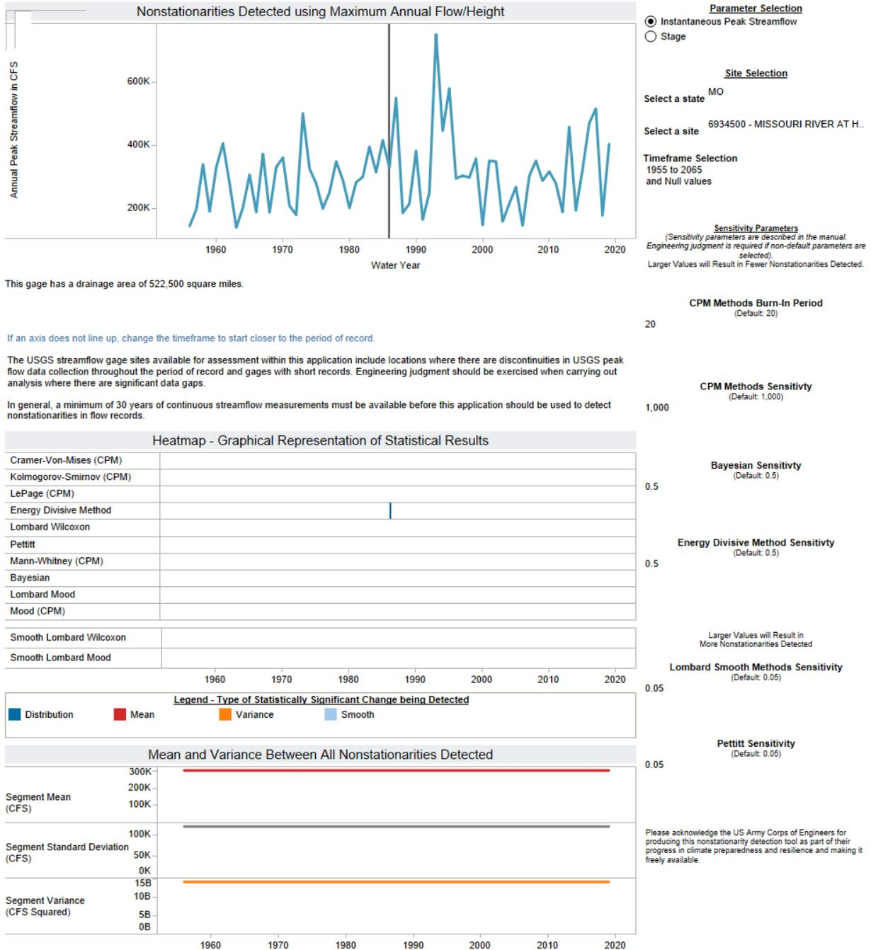
**Figure 39. NSD Output for USGS Gauge 06934500 Missouri River at Hermann, MO**
