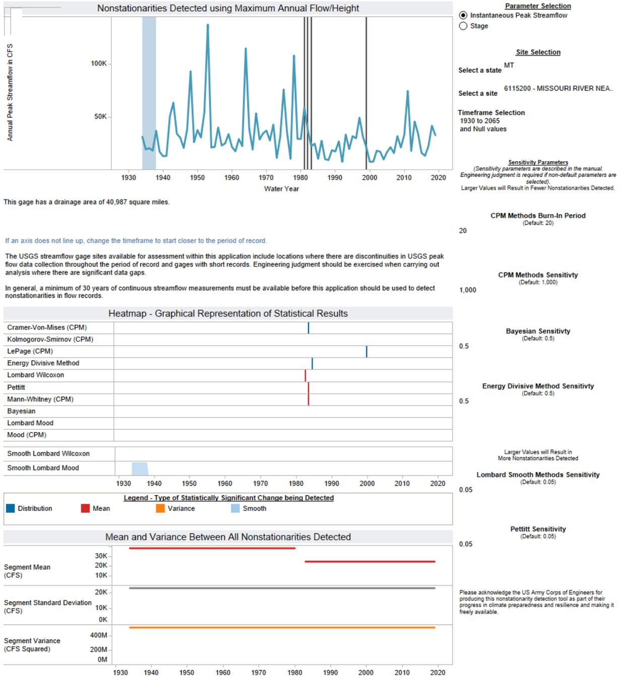
**Figure 33. NSD Output for USGS Gauge 06115200 Missouri River near Landusky, MT**
