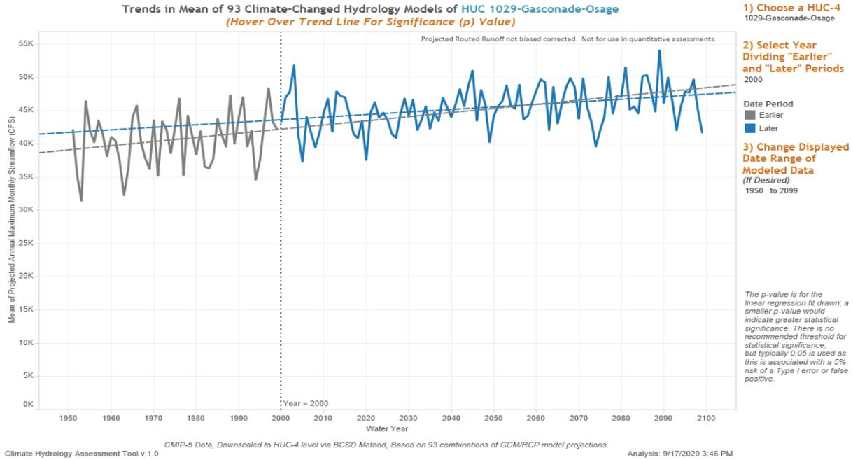
**Figure 39. Linear Regression of Mean Projected Annual Maximum Monthly Flow for HUC 1029 Gasconade-Osage**
