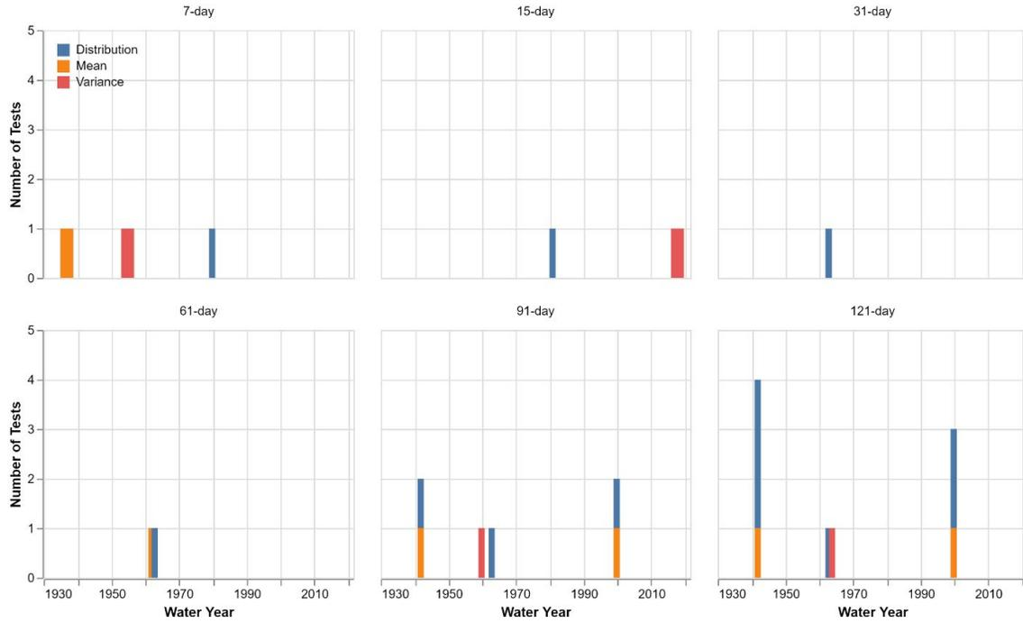
**Figure 52. Big Bend Nonstationary Change Detection Points for n-day Durations Ranging Between 7 and 121 days**
