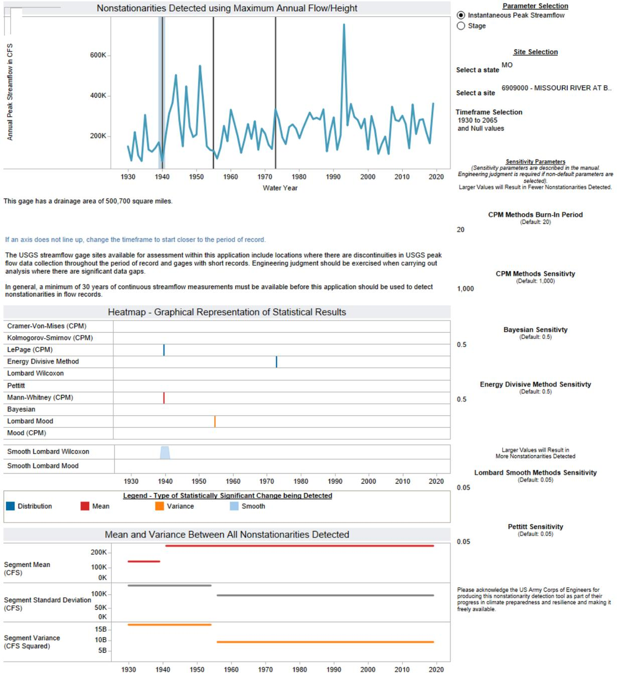
**Figure 38. NSD Output for USGS Gauge 06909000 Missouri River at Boonville, MO**
