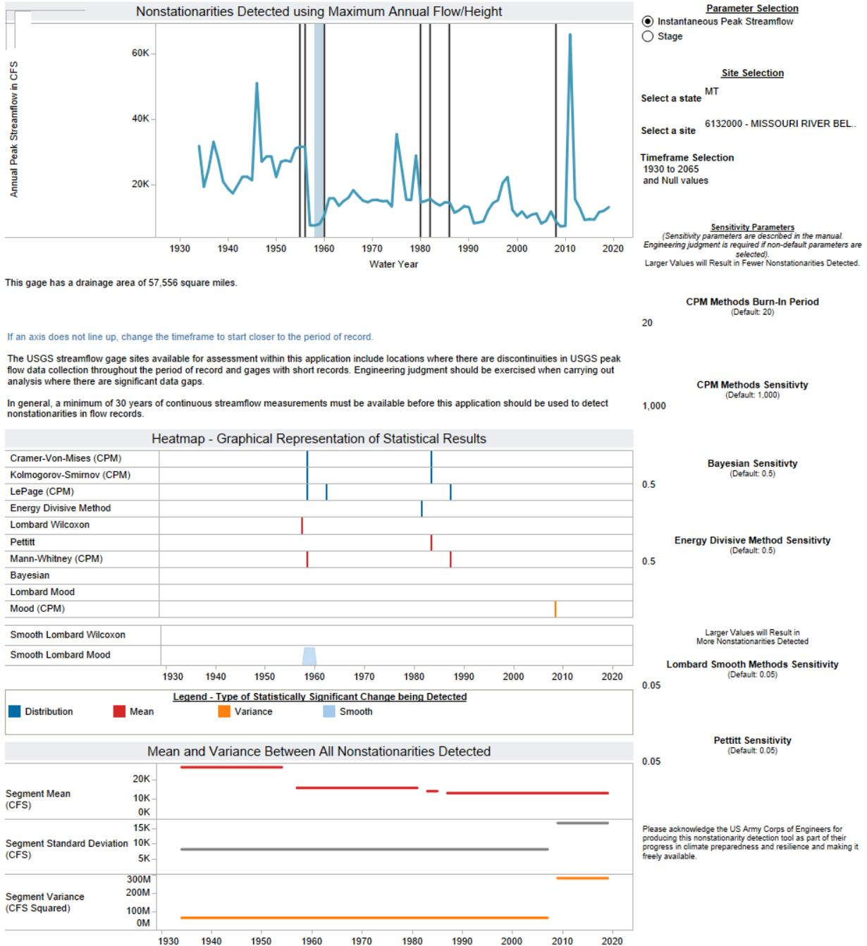
**Figure 31. NSD Output for USGS Gauge 06132000 Missouri River below Fort Peck Dam, MT**
